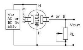
Fig 3.. Electric parameter measurement circuit
