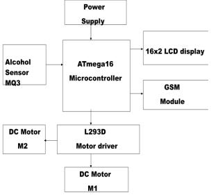
Fig 6. Block diagram of automatic drunken drive avoiding system
